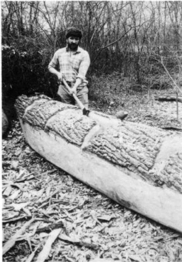
Fig. 4: Removing waste from the top using groove and splinter technique. (Photo: M.A.S.)
