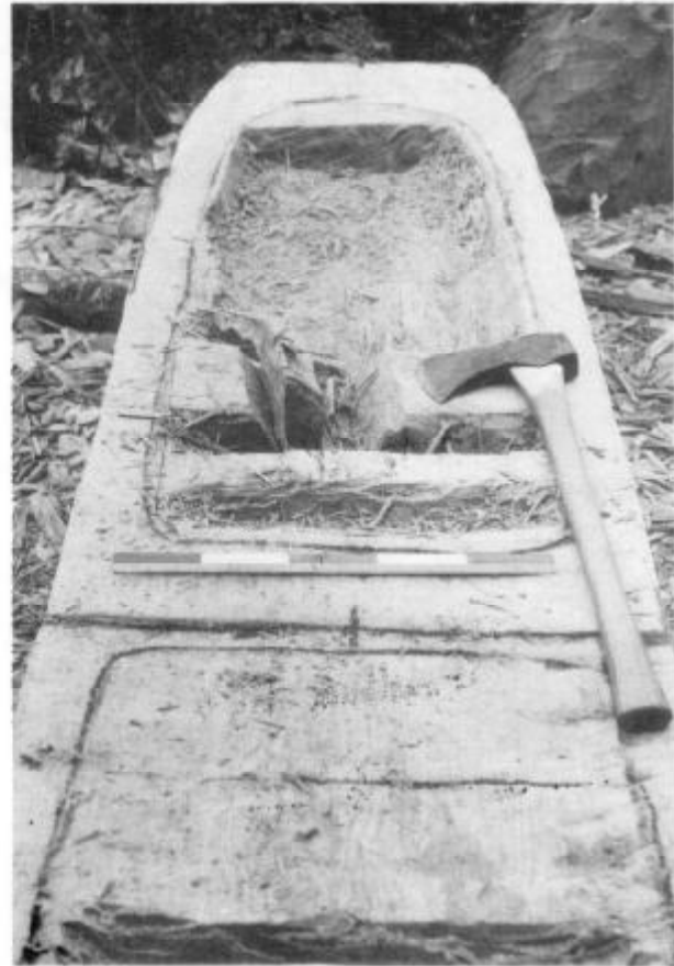
Fig. 5: Hollowing process begun using axe. (Photo: M.A.S.)
