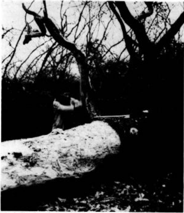
Fig. 2: Day 1, stripping the bark and cross-cutting the log. (Photo: M.A.S.)
